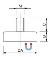
Holdina Part No. ФΑ Μ C В Grade Force (Kg)HM 10 x 4,5 x M4 10 8 4,5 N38 3 4 HM 13 x 4.5 x M5 13 5 8 4.5 N38 6 HM 16 x 4.5 x M6 16 8 4.5 N38 10 6 HM 20 x 5 x M5 5 7 5 N38 20 16 HM 20 x 5 x M5 20 5 13 5 N38 16 HM 25 x 7 x M6 7 27 25 6 10 N38 HM 32 x 7 x M6 32 10 7 N38 6 45
