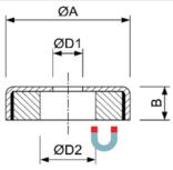
Deep Pot with central Hole Ferrite holding magnet
